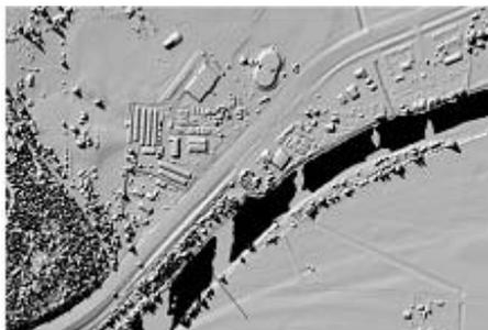
The Orthophotography was flown at 5,100 feet above the average ground elevation and with a photo scale of 1:10,200. A digital orthophoto mosaic having a pixel size of 0.5 ft. and was geo-referenced and scaled to within 1.6 ft. of the points collected with LiDAR. The image was delivered in geo-referenced TIFF and MR SID formats.
