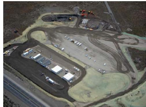
Site preparation consisted of improving and widening the existing access road, and enlarging the existing container transfer area for entire 6 acres. Crews processed over 125,000 tons of material, including on-site excavation material, import gravel, base, and top course. All necessary access roads, facility pads, parking and equipment laydown areas were established.
